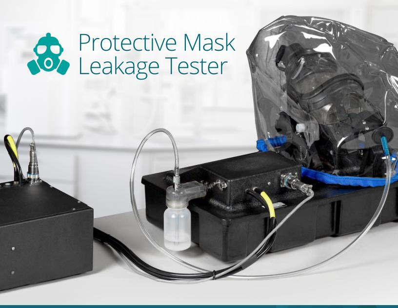
When donning a protective mask, you deserve the utmost confidence in your gear. Air Techniques International's Protective Mask Leakage Tester (PMLT) is an aerosol & photometry-based instrument designed to confirm mask seal and integrity as well as individual fit. The PMLT is portable, easy to use, sets up in minutes and provides a variety of mask testing options.
