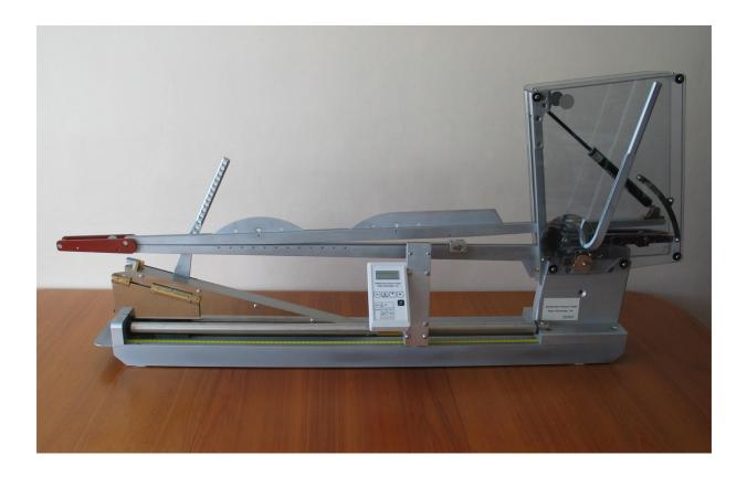
The HATRA Hose Pressure Tester Mk2A+ measures the force exerted by compression hosiery on a simulated leg form to provide hosiery compression values along the leg, and is a development of the Mk2 instrument specified in British Standards BS6612, BS7672, and BS7563.
