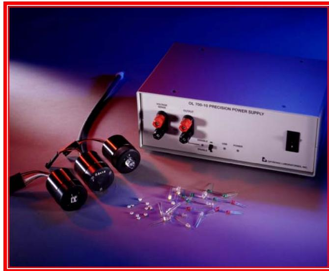
The OL 700-10 Programmable Precision Power Supply offers a lower cost solution to accurately controlling the drive currents of LEDs and small incandescent sources. It is completely controlled by a remote computer via a USB interface.
