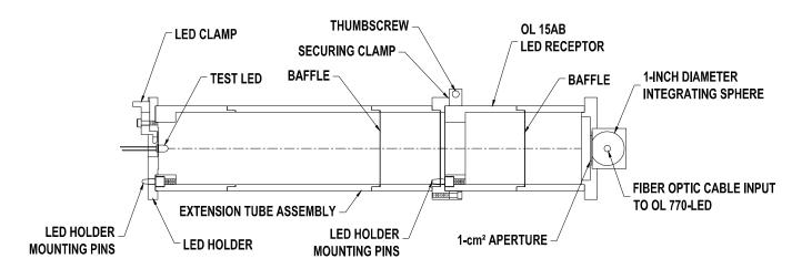
When used with the OL 15 AB, the LED holder snaps into place on either end of the Condition A or Condition B baffle tube. The LED to be tested fits into the mounting hole in the LED holder and is secured in place by a sliding plastic clamp. The LED holder positions the tip of the LED at the correct measurement plane inside the OL 15AB. The LED holder aligns the mechanical axis of the LED with the center of the detector aperture. No other alignment or adjustment is necessary.
