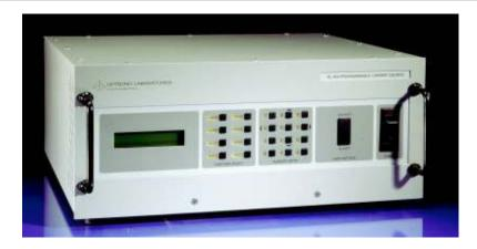
The OL 16A, 65A and 83A are microprocessor controlled, precision DC current sources specifically designed to accurately operate tungsten filament lamp standards and calibration sources. The power output range is 10 to 100 watts for the OL 16A, 10 to 200 watts for the OL 65A and 10 to 1000 watts for the OL 83A. All three units feature:
