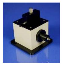
OL 700-73 Solid Transmittance - Utilized for performing spectral transmittance measurements of samples in solid form. Has a slide-in sample holder that accommodates both 1-inch by 1-inch, and 2-inch by 2-inch square samples, as well as 1-inch diameter and 2-inch diameter round samples. Samples can be up to ½-inch in thickness
